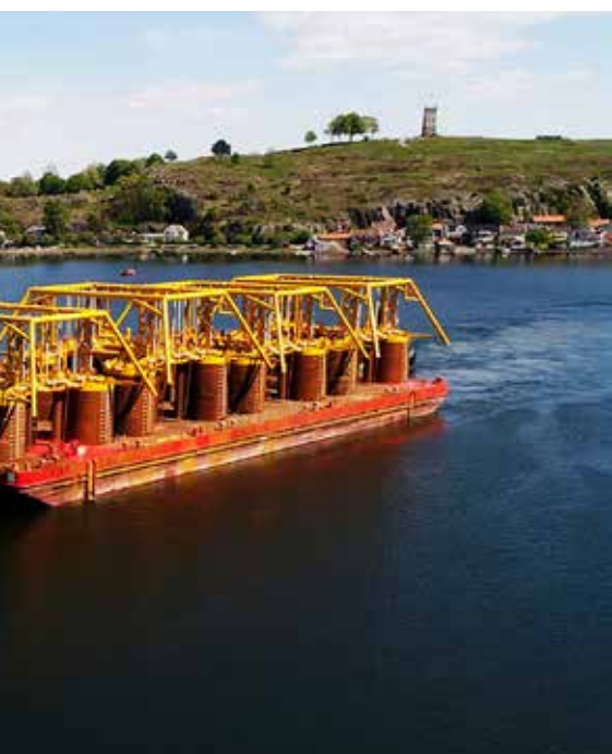
Transport of subsea structures on barge UR 96 for DeepOcean for Equinor's Snorre Expansion Project
